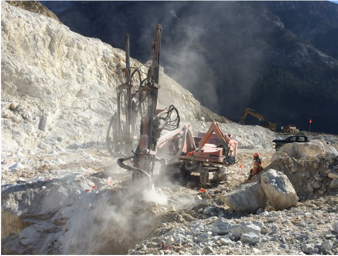
Fig. 14. Blast hole drilling at the Mount Brussilof mine, which produces magnesite from Cambrian carbonate rocks of the Cathedral Formation.
