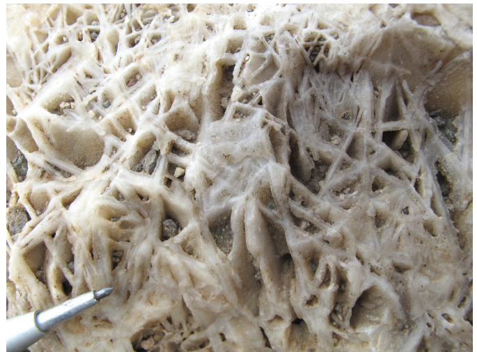
Fig. 16. Trench sample with lattice bladed quartz texture at 2 X Fred.
