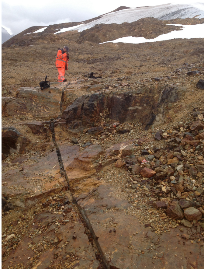
Fig. 16. Channel sampling by Colorado Resources Ltd. on the KSP project near the Tami showing which returned 15 m grading 2.94 g/t Au and 0.51% Cu.
