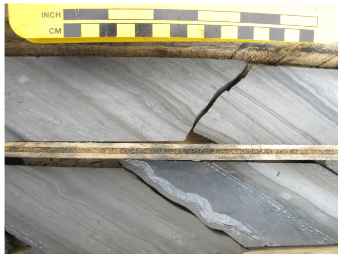
Fig. 13. Akie project, banded sphalerite in drillhole A-15-121.
