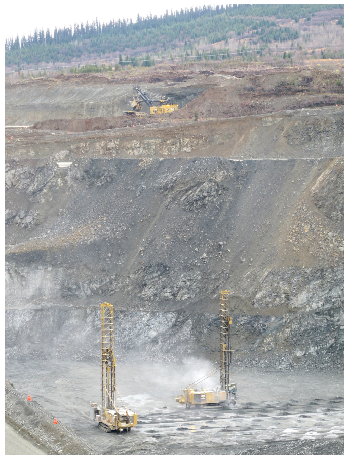
Fig. 9. Blast-hole drilling on the 1010 bench and shoveling on the 1085 bench at Mt. Milligan mine.
