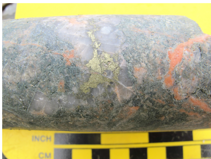
Fig. 19. Quartz-chalcopyrite-pyrite vein in quartz monzonite at Kemess East. Potassic alteration is overprinted by sericite (phyllic) and pink zeolite alteration.
