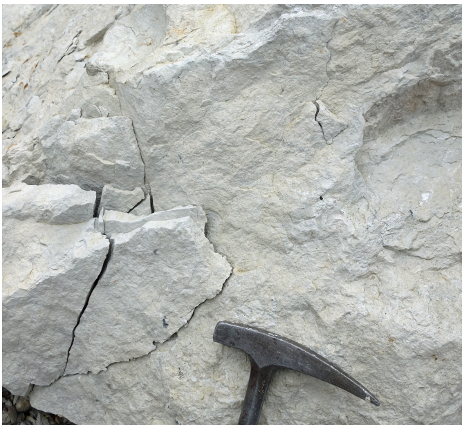
Fig. 9. Intensely altered rhyolite mined as a source of silica and alumina at Electra Stone Ltd.'s PEM 100 quarry.
