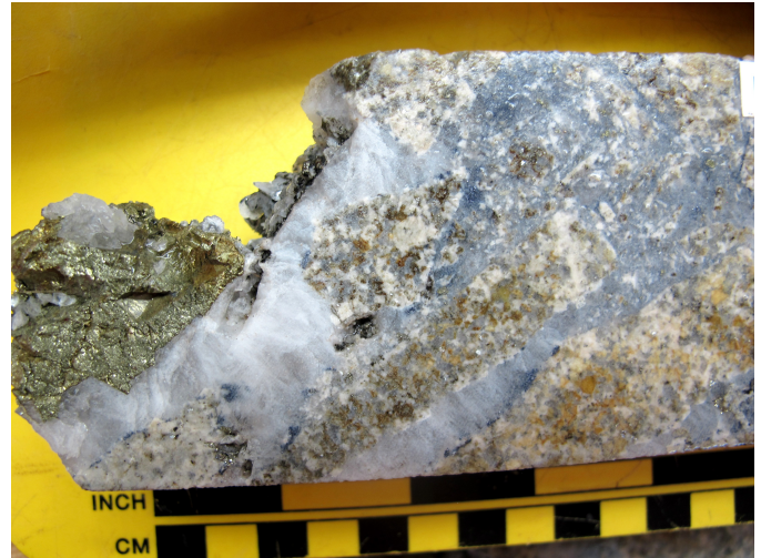
Fig. 13. Quartz-cemented chaotic breccia with disseminated and clotted chalcopyrite-pyrite-molybdenite mineralization in granodiorite at Blackwater South (New Gold Inc., 2015).
