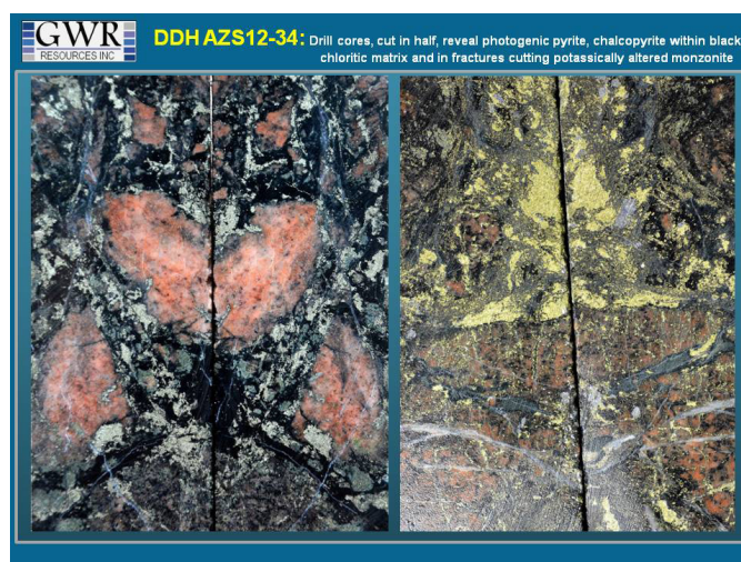
Fig. 6. Breccia textures and copper mineralization at the Aurizon South prospect (Image courtesy of GWR Resources Inc.).
