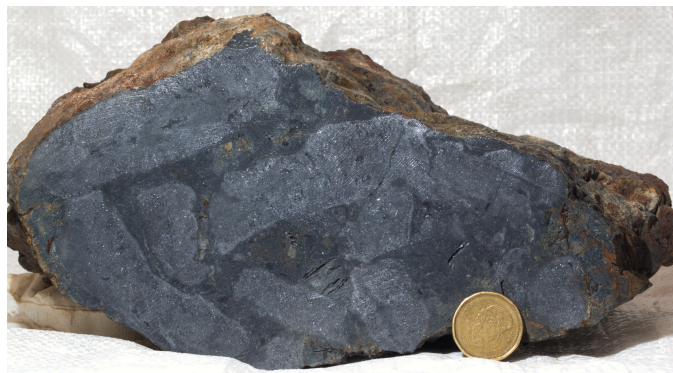
Fig. 18. Hand sample of massive sulphide from the Ace-Galena showing of Dolly Varden Silver Corporation's Dolly Varden Silver project. Photo courtesy of Chris Sebert, Dolly Varden Silver Corporation.
