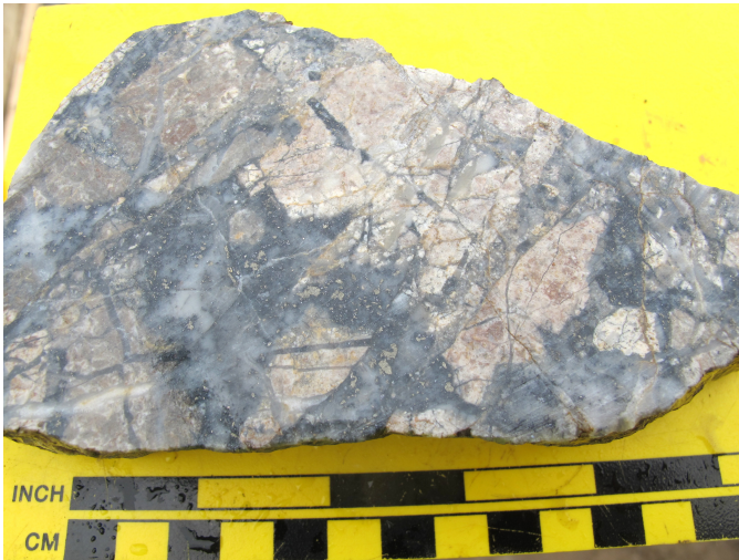
Fig. 17. Slabbed float sample of gold-silver bearing sulphide mineralized multi-stage quartz vein and breccia at Lawyers.
