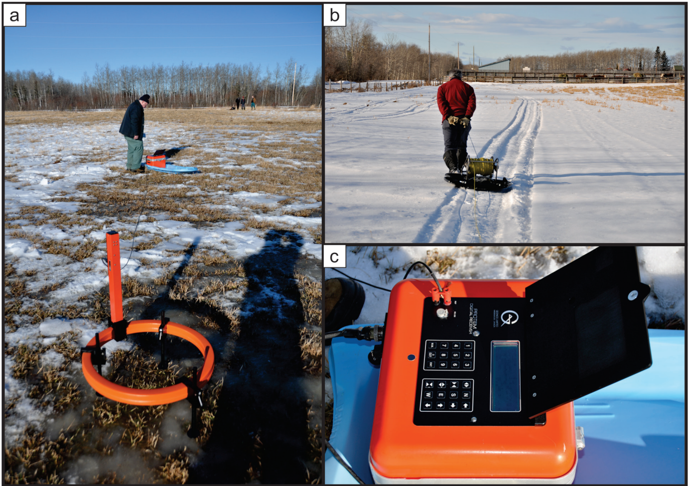
Fig.19. a) EM-47 receiver coil placed in the centre of the large 100 x 100 m loop and connected to the EM-47 control console; b) Laying out the single turn 100x 100 m loop; and c) EM-47 control consol.
