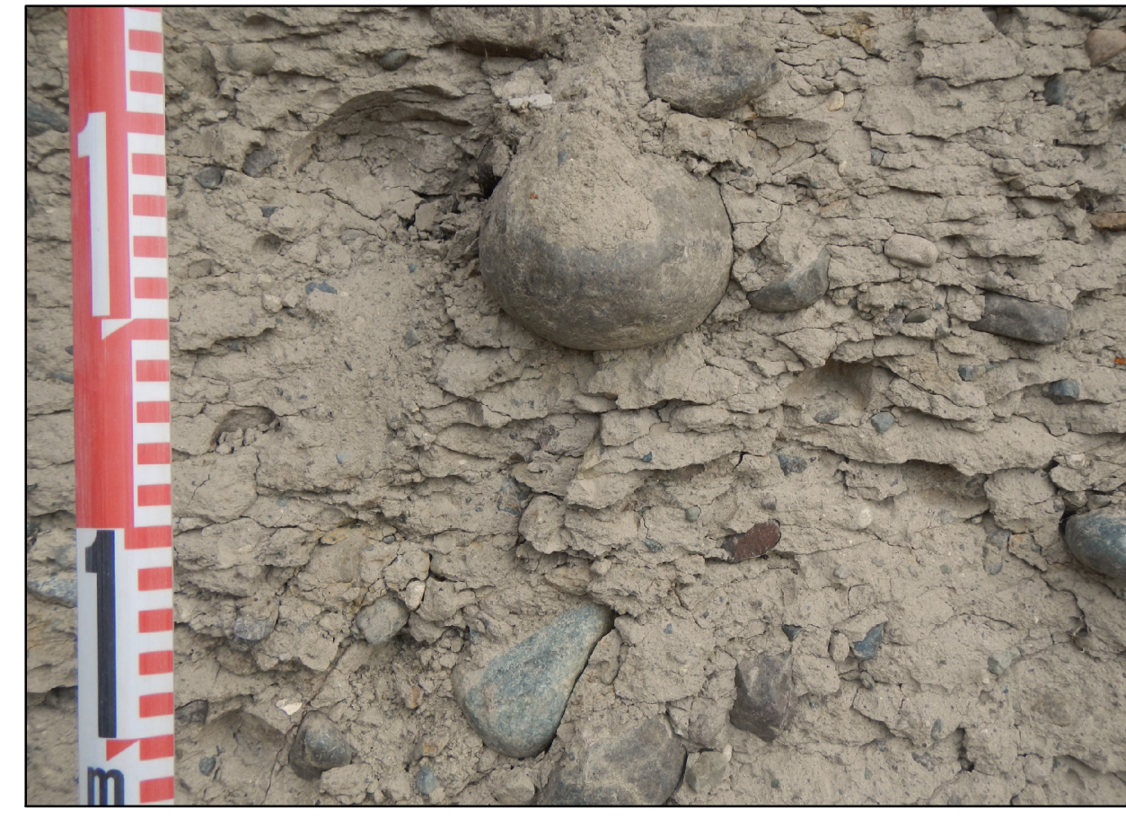
Fig. 2. Basal till in vertical exposure. Note blocky appearance. Granule and coarser-sized clasts float in a clay-silt matrix. Measuring tape in centimetres.
